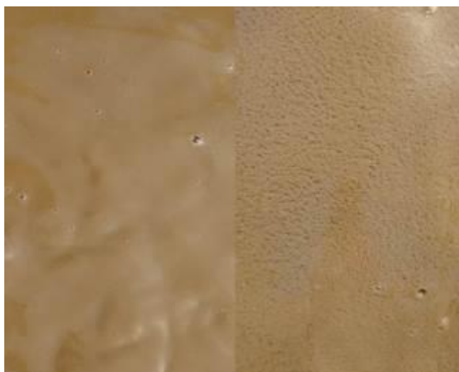
Figure 20. Comparison of the sludge flocculation before and after flux-enhancer addition with activated sludge from the demonstration plant.
